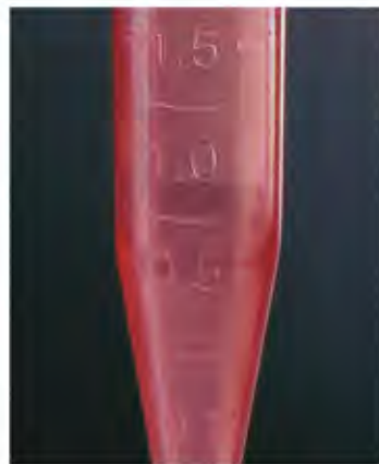
Accurate graduations from 0.1 to 1.5ml provide an easy volume reference
