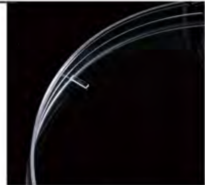
Vents for gas exchange
